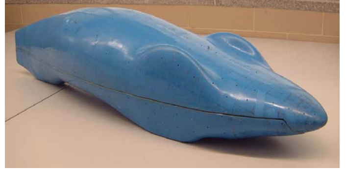
Figure 1 - Model at 1:2.5 scale instrumented with surface pressure taps.
