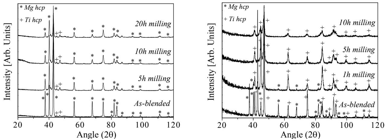
Fig. 1 - X-ray diffractograms of the Ti-Mg powders as a function of milling time. (a)  $Mg_{18}Ti_{82}$ , (b)  $Mg_{50}Ti_{50}$  and (c)  $Mg_{95}Ti_5$ .
