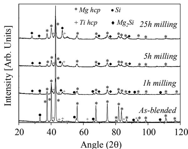
Figure 2 - Structural evolution of the Mg<sub>88</sub>Ti<sub>4</sub>Si<sub>7</sub> mixture with milling time.
