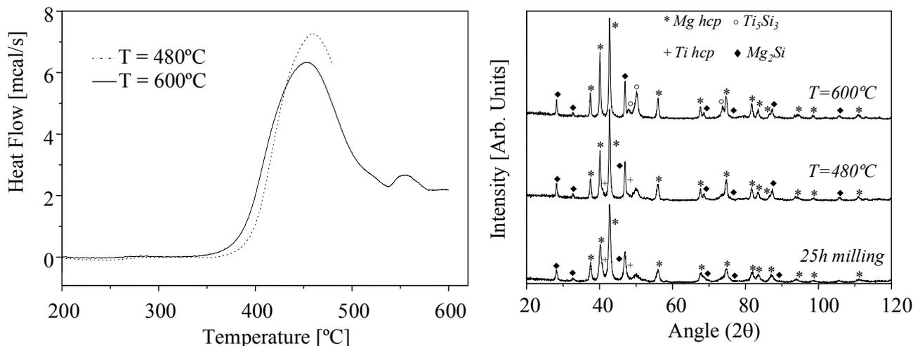
Fig. 3 – (a) DSC curves and (b) x-ray diffractograms of the  $\text{Mg}_{88}\text{Ti}_4\text{Si}_7$  mixture obtained at room temperature after each DSC run.
