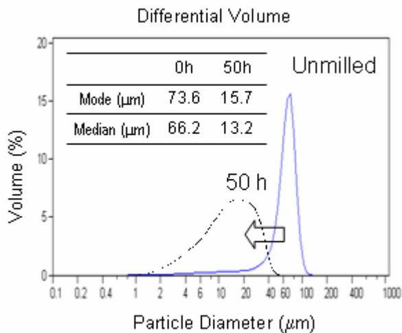
Figure 3 – Particle size distributions of the as-blended and 50 h milled mixtures
