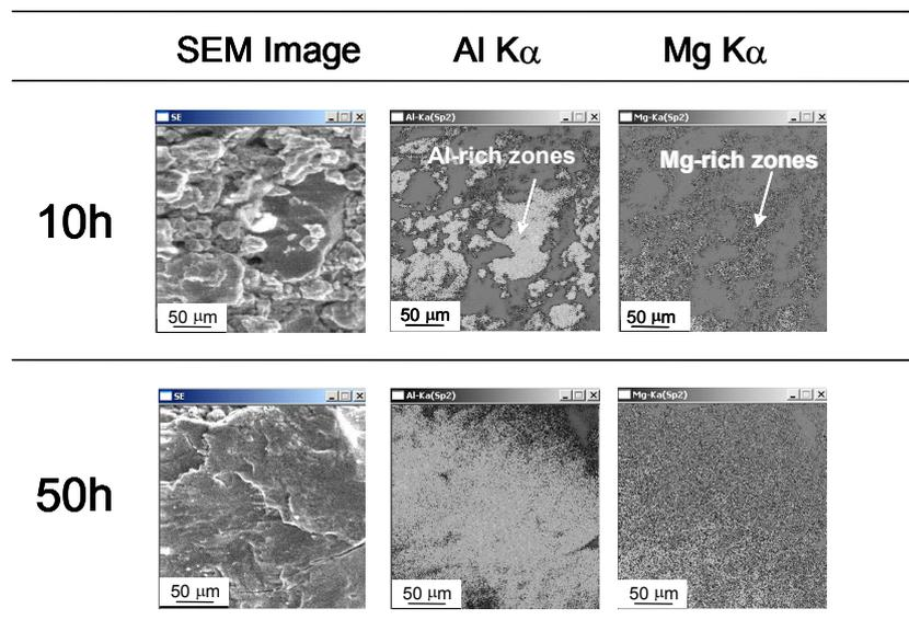
Figure 2 – SEM images and elemental X-ray maps (Al-K $\alpha$  and Mg-K $\alpha$ ) of the Ti-10Mg-5Al mixture after 10 and 50h of milling.
