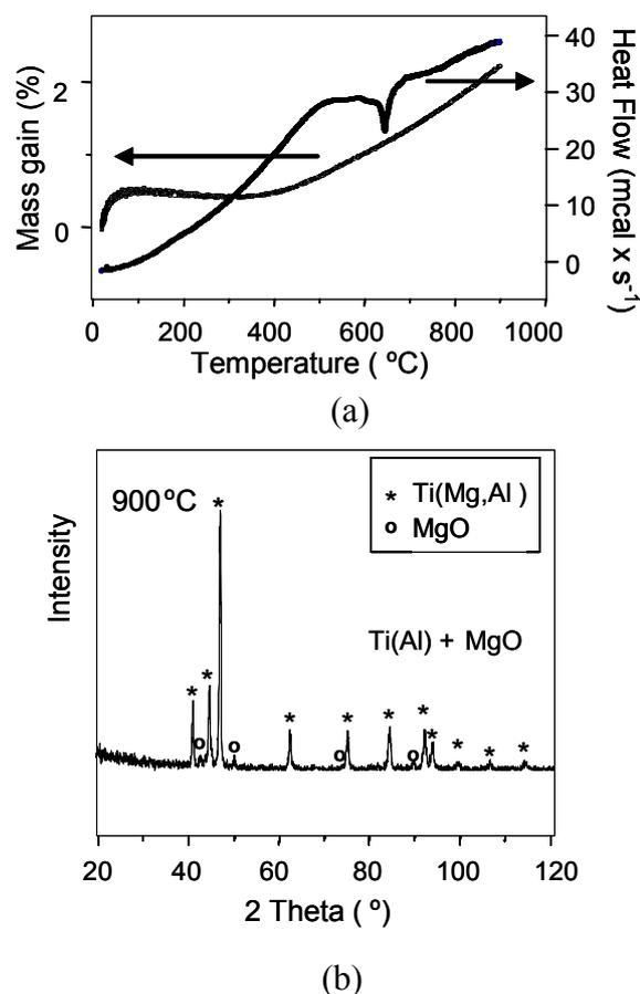
Figure 5 (a) DSC and TG curve and (b) XRD pattern of the Ti-10Mg-5Al mixture.
