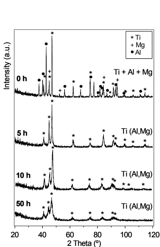
Figure 4- XRD patterns of the Ti-10Mg-5Al mixture as a function of milling time.
