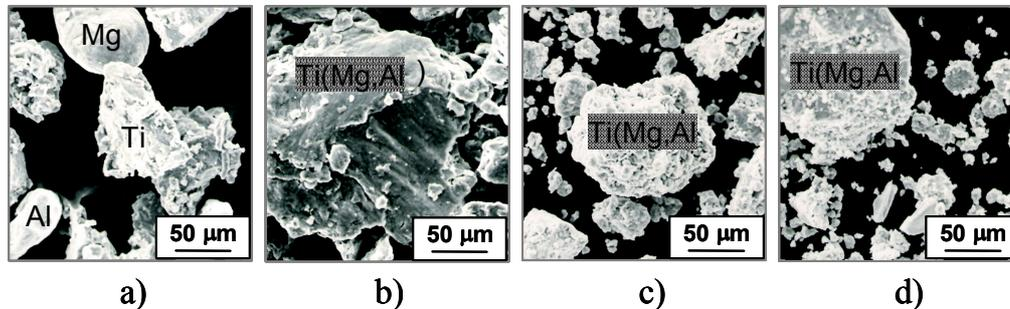
Figure 1 – Scanning electron micrographs of powder particles: (a) as-blended, (b) 5h, (c) 25h and (d) 50h of mechanical alloying
