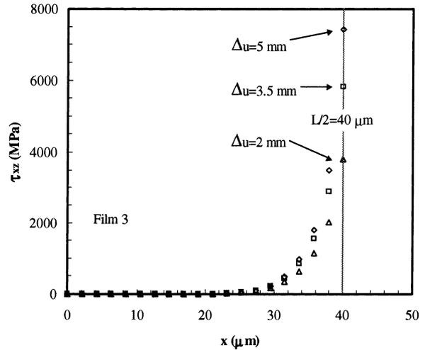
Fig. 10. Shear stress,  $\tau_{xz}$ , distribution along the interface between film 3 and the substrate, for the three displacements used in this study ( $\Delta u = 2, 3.5$  and  $5 \text{ mm}$  and  $L = 80 \mu\text{m}$ ).
