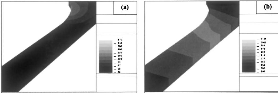
Fig. 5. Distribution at the end of the simulation ( $\Delta u = 5$  mm) of the: (a) shear stress  $\tau_{xy}$  (MPa) and (b) equivalent stress (MPa), for the composite film 1/substrate.
