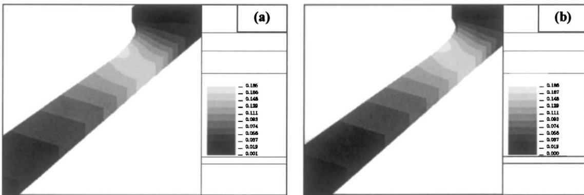
Fig. 6. Equivalent strain distribution at the end of the simulation ( $\Delta u = 5$  mm) for the (a) substrate material and (b) composite film 1/substrate.
