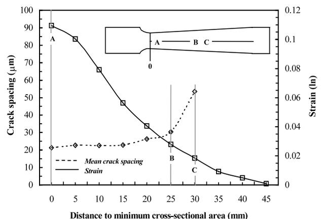
Fig. 2. Experimental results showing the evolution of strain and crack spacing in TiAl films along the axis of the modified sample.
