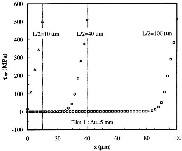
Fig. 8. Shear stress,  $\tau_{xz}$ , distribution along the interface between film 1 and the substrate, for the three lengths of film ( $L = 20, 80$  and  $200 \mu\text{m}$  and  $\Delta u = 5 \text{ mm}$ ).
