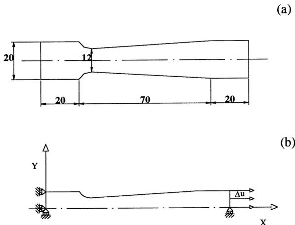
Fig. 1. Continuously variable cross-sectional area sample; (a) tensile test sample (dimensions in mm), (b) boundary conditions.
