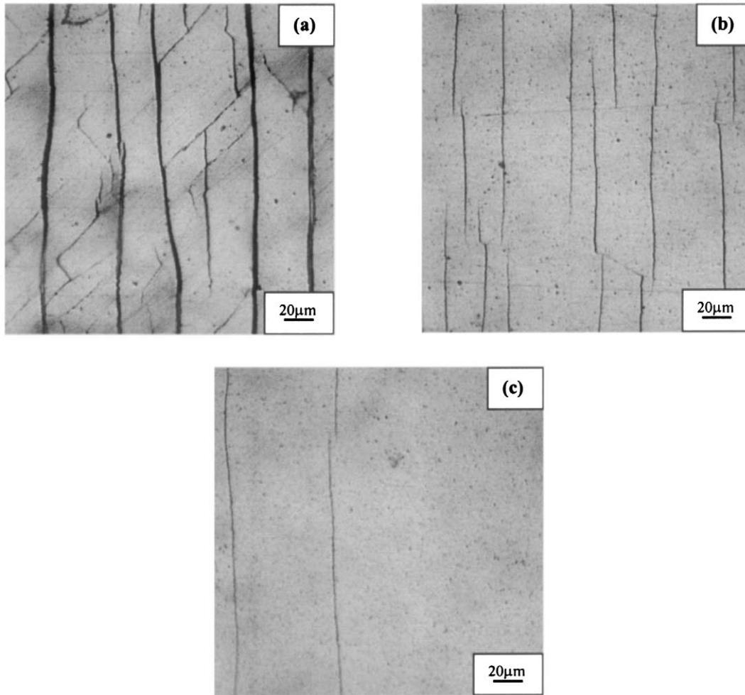
Fig. 3. Optical micrographs showing cracks in the TiAl films at different strain values, for region A, B and C of Fig. 2, respectively: (a)  $\varepsilon = 0.11$ ; (b)  $\varepsilon = 0.03$  and (c)  $\varepsilon = 0.02$ .
