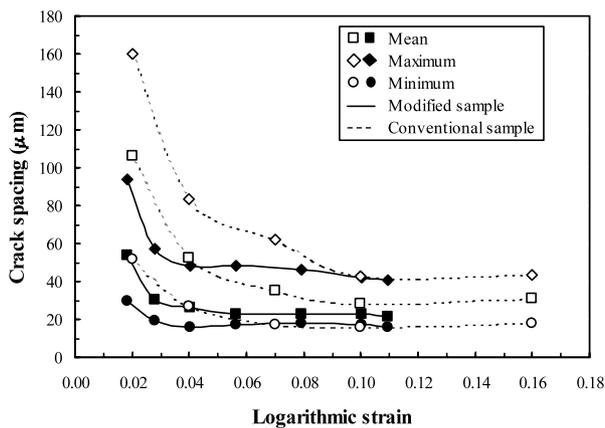
Fig. 4. Example of the evolution of the mean, maximum and minimum crack spacing with deformation, for modified tensile samples. The evolution of the mean, maximum and minimum crack spacing with deformation for conventional tensile samples is also shown. Experimental results obtained in TiAl films deposited onto stainless steel substrates. Only distances between cracks normal to the symmetry axis were measured.
