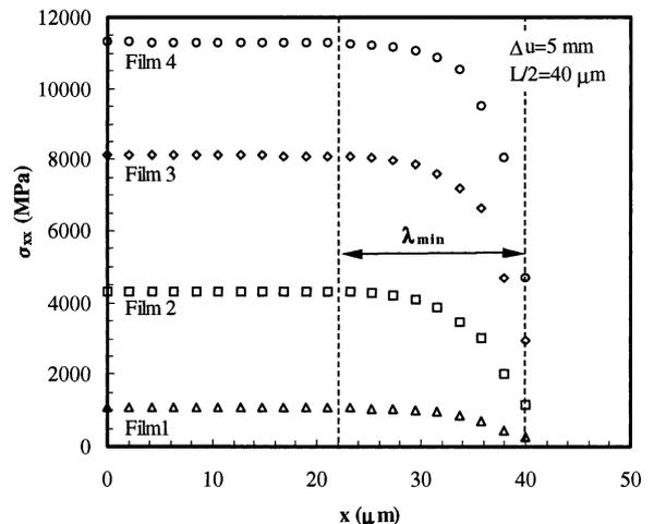
Fig. 11. Tensile mean stress,  $\sigma_{xx}$ , distribution along the interface film/substrate for the four film materials used ( $L = 80 \mu\text{m}$  and  $\Delta u = 5 \text{ mm}$ ).
