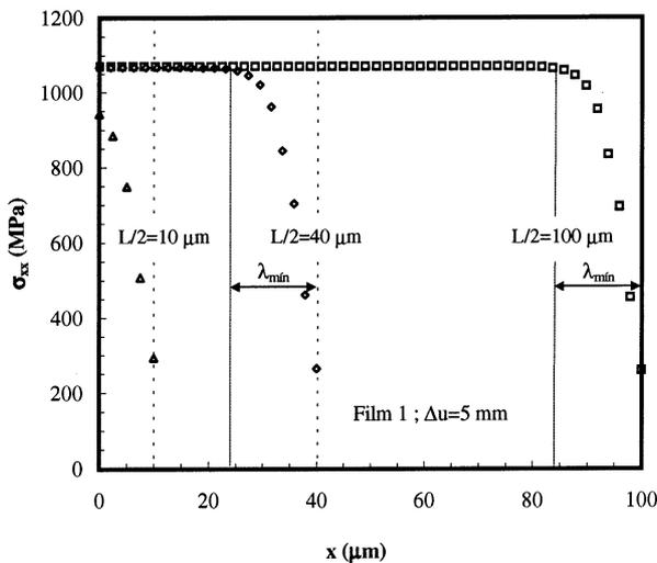
Fig. 9. Tensile mean stress,  $\sigma_{xx}$ , distribution along the interface between film 1 and the substrate, for the three lengths of film ( $L = 20, 80$  and  $200 \mu\text{m}$  and  $\Delta u = 5 \text{ mm}$ ).
