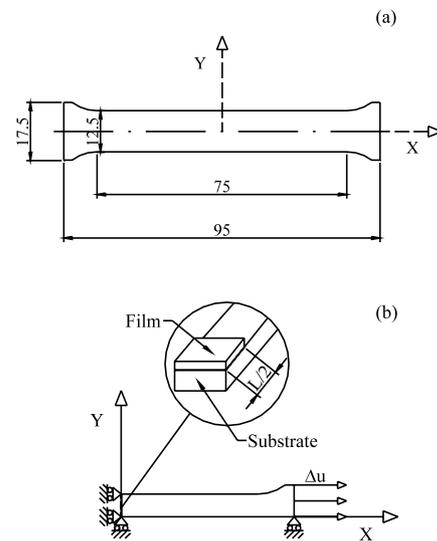
Fig. 7. Conventional tensile test sample used in the simulations with a thin film: (a) sample geometry (dimensions in mm); (b) boundary conditions for the numerical sample and details of film plate in the central region of the sample.
