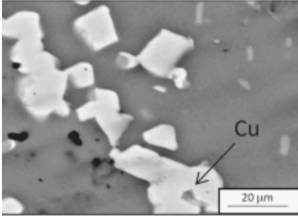
**Fig. 5.** Morphology (BSE-SEM image) of the Ti-35Si-10Mg-Cu HIP'ed sample showing segregation of Cu.
