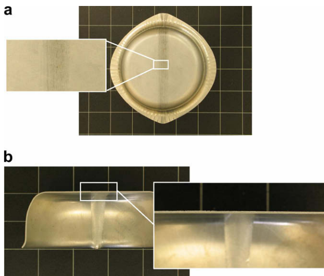
Fig. 10. Magnifications of the weld roots of the S66-D20 (a) and S55-D18 (b) cups.
