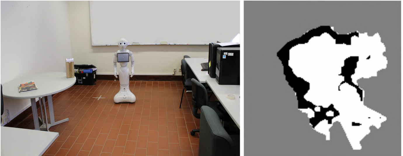
Fig. 2. Real environment (left) and resulting map representation of the explored area (right).
