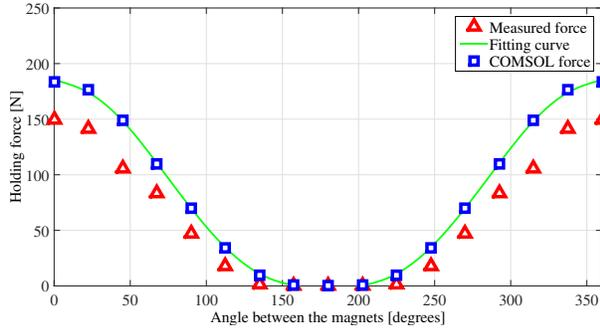
Fig. 7. Variation of the holding force according to the moving magnet's angle.
