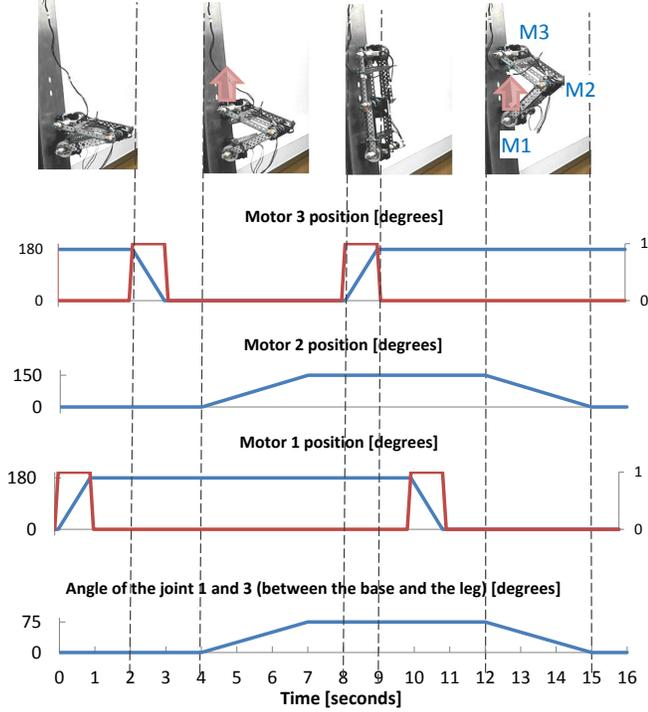
Fig. 10. Motor gaits and joint positions during a full climbing cycle. Blue shows the motor position and red shows the power input to the motor. As can be seen the power input to switchable magnet units is only during switching action
