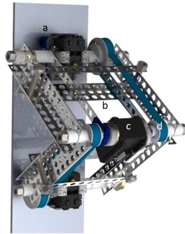
Fig. 1. InchwormClimber: a- Adhesion Unit with actuator, b- transverse bar, c- climbing mechanism actuator, d- pulley and belt.
