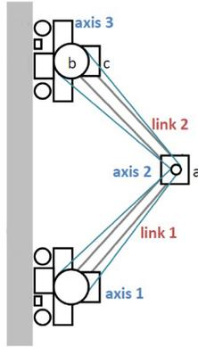
Fig. 8. Side view schematics: a- Climbing mechanism actuator, b- Pulley, c- Adhesion unit.
