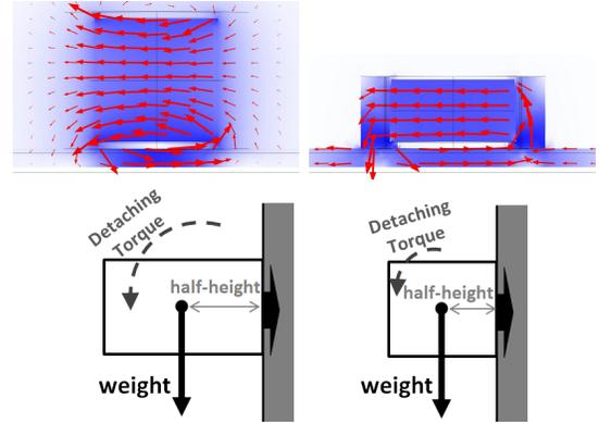
Fig. 6. Above: Simulations in *Comsol Multiphysics*. Below: Reduction of the detaching torque with a lower profile.
