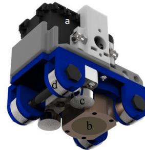
Fig. 3. Adhesion unit: a- AX-12 actuator, b- switchable magnet, c- permanent magnet, d- bearing.
