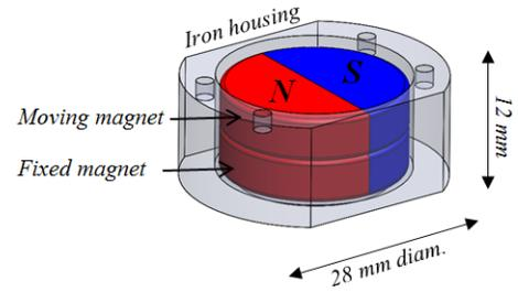
Fig. 5. Novel optimized switchable magnet unit.
