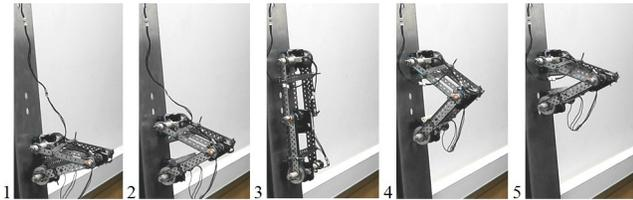
Fig. 11. InchwormClimber climbing during experiments.
