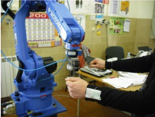
Fig. 1. Industrial robot MOTOMAN HP6 controlled by arm gestures and postures.
