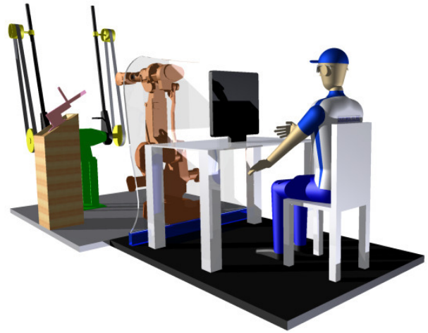
Figure 1. Off-line robot programming concept. Working in an office environment, the user can generate robot programs without interrupt production.
