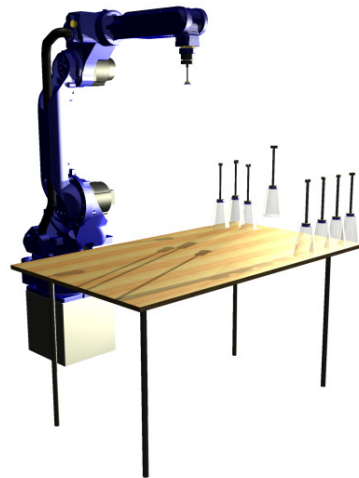
Fig. 3. CAD assembly model of the robotic material handling cell. A robot program will be generated from this CAD model.
