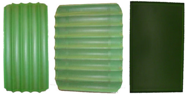
Fig. 6 Three different workpieces produced by FLUPOL. Horizontal wavy-surface plate (left), vertical wavy-surface plate (middle) and smooth surface (right)
