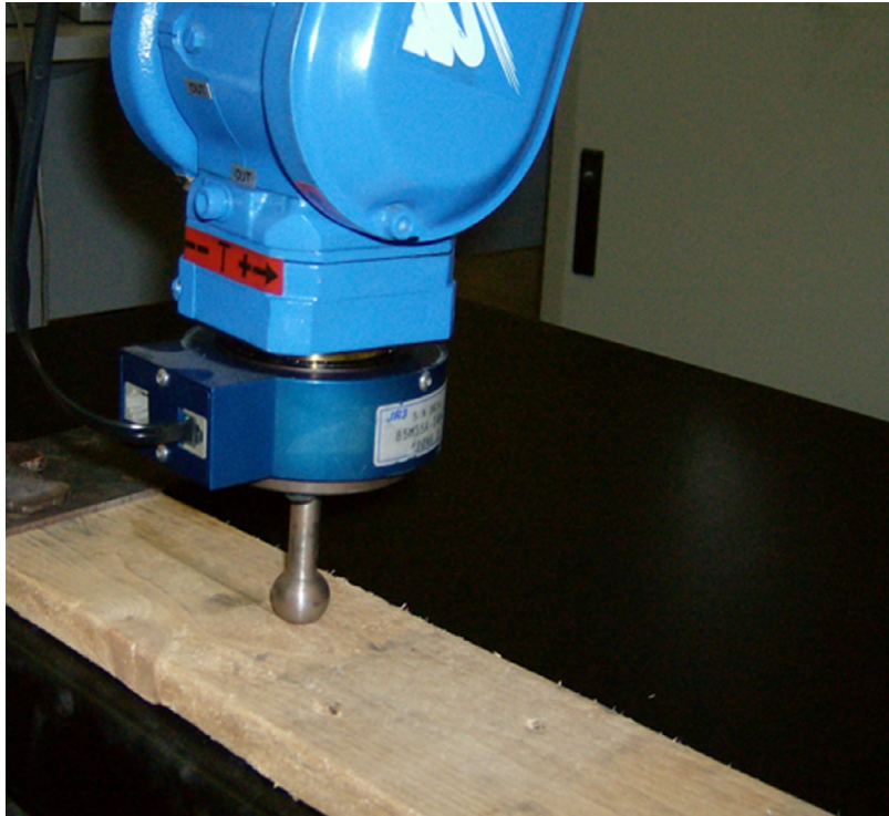
Fig. 3. Robot end-effector in contact with a pine wood work piece.
