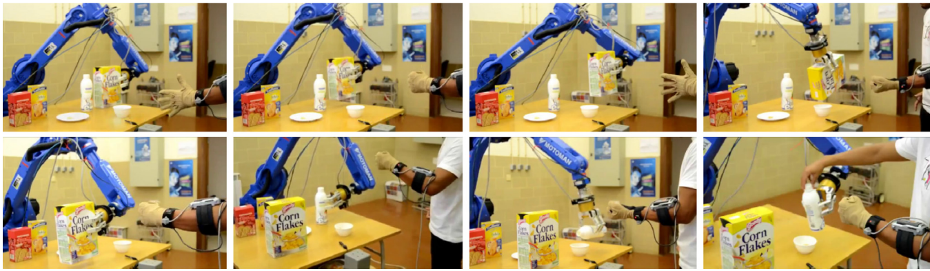
Fig. 8. Visualization of different stages of robot teleoperation process: (a) starting point, (b) virtual joystick guidance to a goal, (c) forceful stop command, (d) rotation of the end-effector, (e) gesture-command to open the gripper, (f) grabbing a bottle and pulling it up, (g) rotation of the end-effector, (h) safe collaboration with the robot. NOTE: The virtual joystick mode moves the end-effector in a direction defined by the vector that joins a center position in which the hand is closed and the position of the hand when it is moved.
