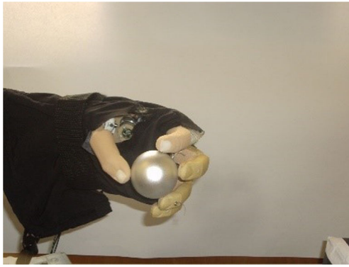
Fig. 1 The ISR-Softhand grasping a spherical object. The exerted forces cause undesired deflections on the compliant joint of the thumb, affecting the grasp stability. Grasping heavier objects is impossible, even if the thumb can exert enough normal force
