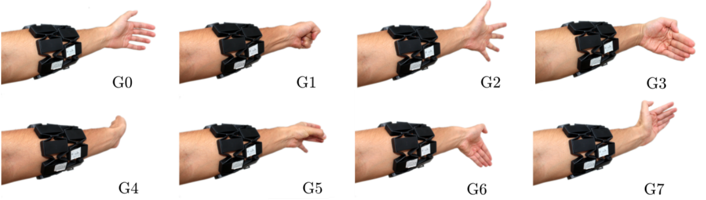
Fig. 2. UC2018 DualMyo dataset gestures: (G0) rest, (G1) closed fist, (G2) open hand, (G3) wave in, (G4) wave out, (G5) double-tap, (G6) hand down, (G7) hand up.
